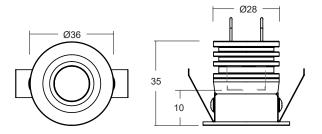
IP54 rated version is supplied with an extra gasket which sits between the bezel and the mounting surface.
